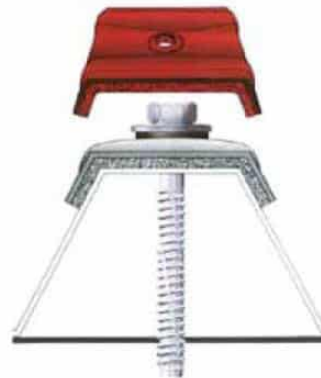
Picture 41. Connector with calotte - assembly in the hump of the roof panel.
